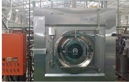
Low Liquor Dyeing and Washing Machine (Installed in C&T G-Tech)
