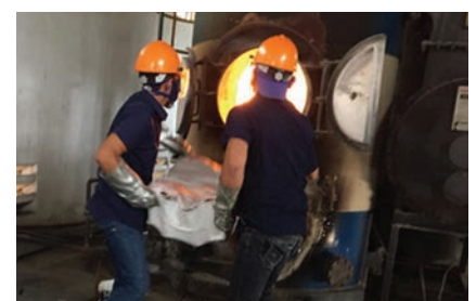
Incinerator Burning Biomass
